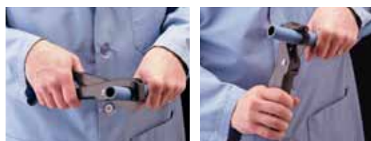
The rotating/rocking technique produces fast easy cuts.
